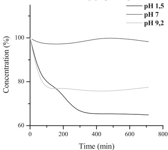
**Fig. 2** Time dependence of the measured absorbance at 282 nm for the model compound solution in Series 1 (pH=1.2), Series 2 (pH=7.4) and Series 3 (pH=9.0).
