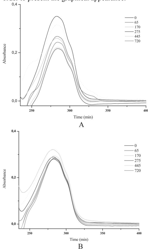
**Fig. 1** The corresponding UV/VIS spectra recorded for the relative aliquots of the model compound at 37°C and pH=1.2 (A) and pH=7.0 (B) at the specified time intervals.
